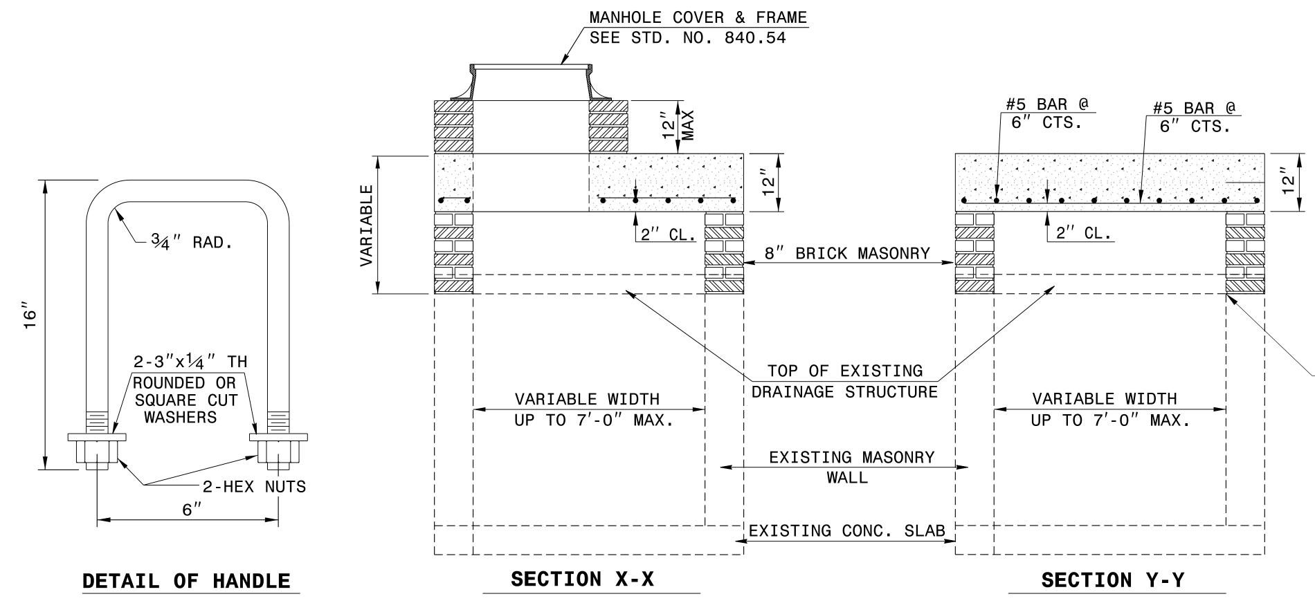
ALIGN PROPOSED BRICK VERTICAL ADJUSTMENT TO INNER FACE OF WALL
